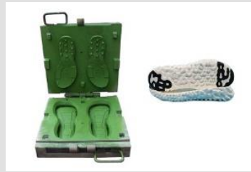
Co-molding Process of EVA & Rubber Sole
