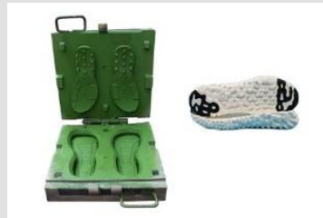
Co-molding Process of EVA & Rubber Sole
